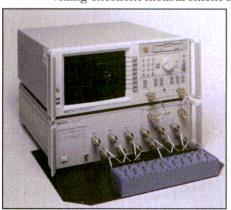
1. An Agilent 8712E series VNA and Agilent 87050E multiport test set form a complete 50- $\Omega$  multiport test system.
