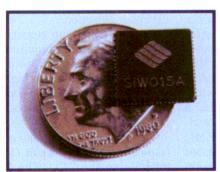
1. Less than 1-mm thick, Silicon **Wave's Bluetooth integrated** circuit (IC) combines radio. modem, and controller functions in a single component.
