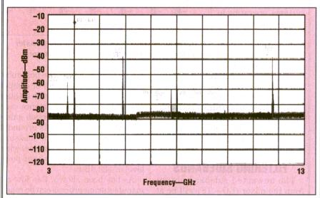
9. These measured results show the output spectrum of the downconverter's IF port, using an RF input signal at -40 dBm.
