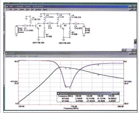
This split-screen view shows LINC2's schematic capture and simulated performance-display capabilities.
