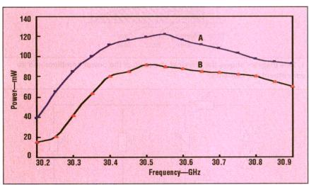
3. This graph shows the power output versus frequency of the individual Gunn diodes when activated separately.
