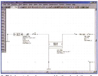
2. This input signal was used in the simulation. A +1.5-VDC offset was used for each of the voltage source elements in order to achieve a 0-V gate-source voltage for each PHEMT driver.
