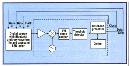
This BER test setup employs output signals from the Bluetooth DUT's baseband processor.
