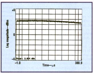
division systems, such as 3. This display of average and peak power was made with an HP 89441A VSA at 2.402 GHz using a sweep time of 380  $\mu$ s.
