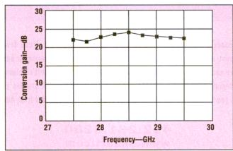
Option 1 is not the best 8. The conversion gain of the frequency downconverter approach for low-cost, high- was measured around 23 dB as a function of frequency.
