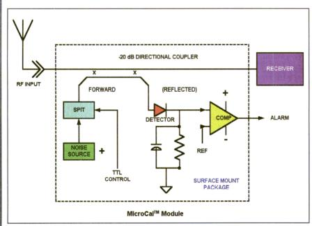
1. This block diagram shows an example of a MicroCal noise module integrated with a SPST switch and dual directional coupler.
