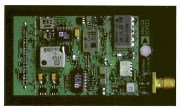
data GSM environment The AD6523 and AD6524 ICs from Analog Devices show (EDGE) and general-pack- how a direct-conversion architecture occupies a small amount of circuit-board area.
