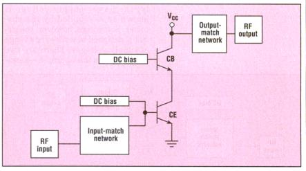
3. This block diagram illustrates the two-transistor cascode configuration, along with the DC bias and impedance-matching networks.
