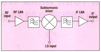
bond for 0.001-in.-diameter 6. The millimeter-wave frequency downconverter module Au bond wire. At lower fre- is designed to handle input frequencies from 27.5 to 29.5 quencies, the reactance that **GHz and provide an IF of 4 GHz**.
