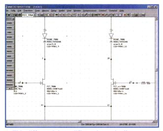
1. This differential amplifier schematic diagram was developed with the MMICAD WAVEFORM program.
