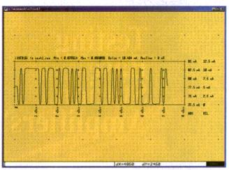
4. This is the current waveform that was used to drive the differential amplifier's right-side laser diode, as viewed by MMICAD WAVEFORM's voltage probe.
