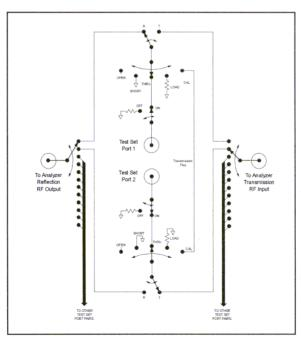
whereas calibrating all possible 3. This simple block diagram shows one pair of paths of a three-port device usinternal calibration standards within the ing a traditional VNA requires Agilent 87050E multiport test set.
