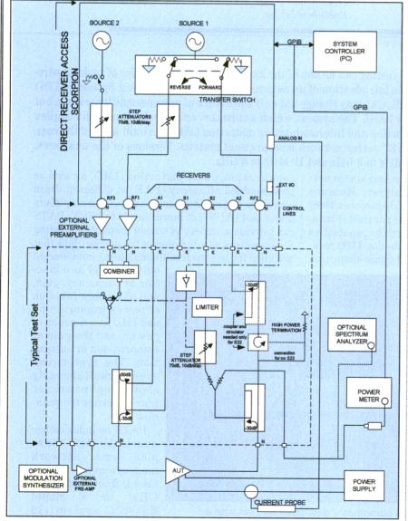
2. The basic architecture of PATS consists of a Scorpion VNA with direct-receiver-access (DRA) capability, a dedicated test set, and measurement software on a PC connected through GPIB.
