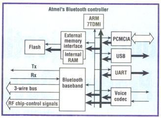
2. Atmel's AT76C551 Bluetooth controller, available in several options, integrates an ARM7TDMI core and dedicated Bluetooth baseband block.
