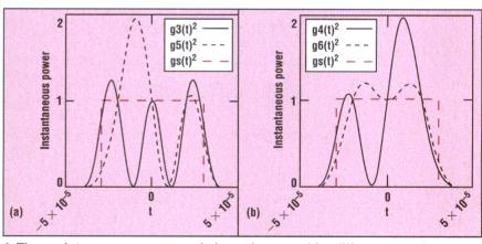
4. The peak-to-average power ratio is not increased for different combinations of three consecutive RRC pulses. Two combinations, g5(t) in (a) and g6(t) in (b), produce the same peak value. Calculating the average value for each sequence provides almost equal results. The resulting peak-to-average ratio is very close for both sequences.
