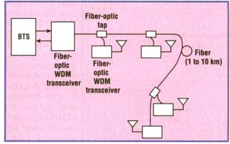
4. An optical tap is intrinsically bidirectional, allowing it to couple signals from and insert signals into a fiber-optic link.
