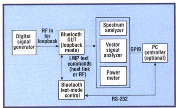
This measurement setup is suitable for evaluating the performance of Bluetooth transmitters. If a direct cable connection is not available between the Bluetooth DUT and the test equipment, a coupling device (such as an antenna) is needed. control. Since cable losses and impedance mismatches within the Bluetooth band can be severe, good-quality interconnections and components should be used as part of the test setup.
