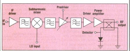
10. The frequency upconverter is based on a heterodyne architecture using commercially available components.
