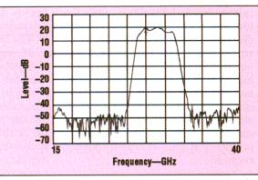
$\mu$  m - g a t e - l e n g t h 11. These plots show the measured nominal gain of an MMICs, upconverter subcircuit containing the predriver used in bare die form. amplifier and two printed coupled-line bandpass filters.
