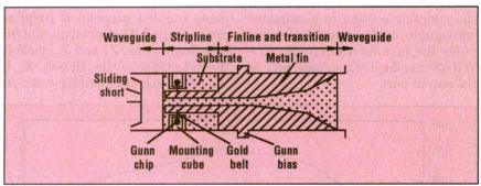
1. This diagram shows the physical structure of the power combiner and its constituent components.
