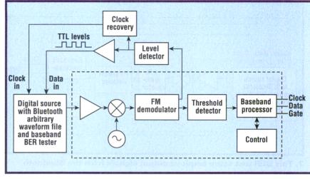
8. This modification to the BER test setup uses the output of the Bluetooth receiver's FM demodulator.
