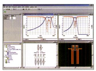
2. The software's multifunction capabilities support a single screen with schematic diagram (lower left), layout (lower right), and simulated performance (upper plots).
