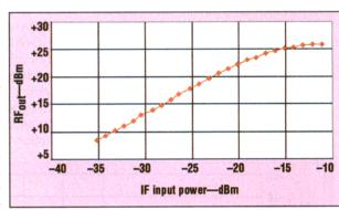
stant-envelope modu- 12. These plots show the measured power-transfer lation schemes and characteristics of entire frequency upconverter.
