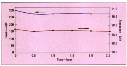
5. This graph of the power output and frequency of the combiner demonstrates its stability over two 2.5-h periods.
