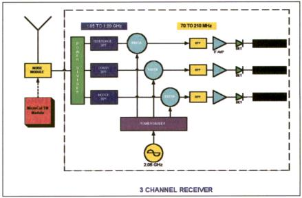
3. This three-channel receiver was simulated with SystemView software to demonstrate the effectiveness of the MicroCal noise modules.
