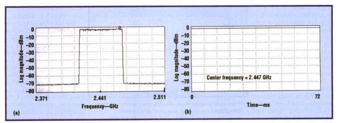
4. These displays of power density were made with an HP 8594E spectrum analyzer at a center frequency of 2.441 GHz and span of 240 MHz (a) and center frequency of 2.477 GHz and span of 0 Hz (b).
