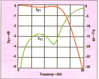
strate, minimizing the 5. This simulated performance is based on the model of a lengths of bond wires (and lowpass filter structure incorporating the 0.3-nH the resulting parasitic inductance of a typical Au bond wire.
