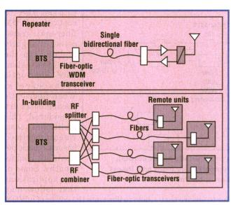
2. These are only two examples of system configurations for a fiber-optic-based RF transmission and distribution system.
