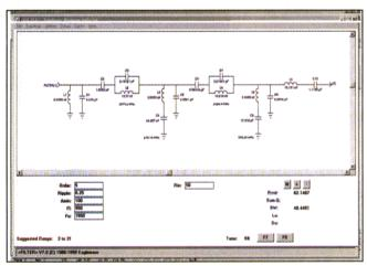
1. GENESYS 7's lumped-element design screen was used to develop this multistage filter.
