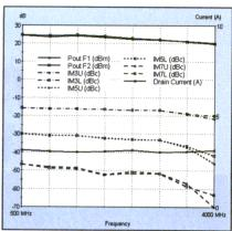
3. An example of the many measurements available with PATS are these output-power and IMD measurements made as a function of frequency. Similarly, gain, harmonic distortion, and PAE can be measured for a particular saturation or compression point.
