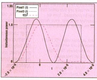
2. Two consecutive RRC pulses can have opposite polarities (shown here) or the same polarity (see Fig. 3). The curves represent the instantaneous power (Pinst1) for the sequence compared to two consecutive square pulses (Pinst3).
