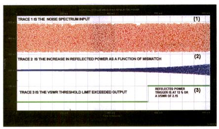
2. These three traces show the noise input spectrum (top), the increase in reflected noise power from a power impedance match (middle), and the VSWR threshold trigger (bottom).
