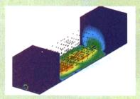
FIDELITY modeling of a cylindrical dielectric resonator and the Poynting vector display
