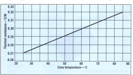
3. This graph shows the maximum thermal resistance versus case temperature for the SD2923.
