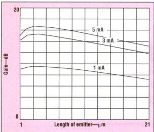
2. This graph shows the change in performance of the single-transistor, common-emitter LNA as the emitter length varies.
