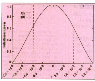
1. A square unshaped pulse (dashed line) is shaped by a root-raised-cosine function (solid line) into an amplitudemodulated signal. Shaping is necessary to distinguish between symbols to improve system performance.
