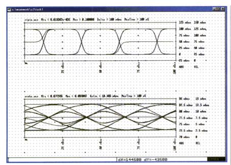
These eye diagrams were generated for the differential amplifier simulated at 40 Gb/s.
