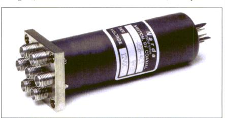
This SP6T coaxial switch provides low loss and high isolation through 18 GHz and is designed to fit in a single-slot C-size VXI card format.
