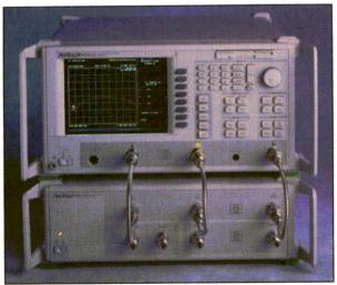
measurements, includ- 1. PATS combines a dedicated test set with a ing all four S-parame- powerful vector network analyzer (VNA) and ters (including "hot" S22 measurement software to automate once-difficult measurements), gain nonlinear amplifier measurements.
