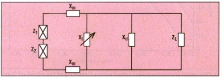
2. This schematic diagram shows the power combiner's equivalent circuit.
