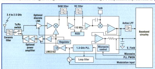
1. This block diagram shows a complete Bluetooth transceiver based on the LMX3162 IC.
