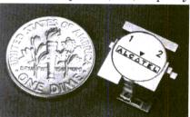
band of 1930 to 1990 MHz. Isolation is specified at 20 dB minimum, insertion loss is 0.4 dB maximum, VSWR is 1.25:1, and phase flatness is 0.3 dB, peak-to-peak. The isolator comes in a package measuring  $0.44 \times 0.50 \times 0.25$  in. ( $1.12 \times 1.27 \times 0.64$  cm). The operating temperature range is 0 to 85°C. Alcatel Ferrocom Ferrite Products, 6385 San Ignacio Ave., San Jose, CA 95119; (408) 229-8171, FAX: (408) 229-8506, e-mail: s a l e s f e r r o c o m@a u d . alcatel.com.
