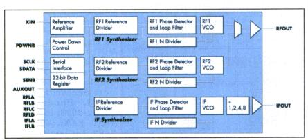
All the functions necessary to perform dual-band synthesis for high-speed wireless data are contained on a single 0.35- $\mu$ m CMOS chip, the Si4133G from Silicon Laboratories.
