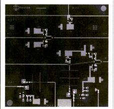
1. This photograph shows the millimeter-wave downconverter MCM. All decoupling was realized through 0402-size SMT components.
