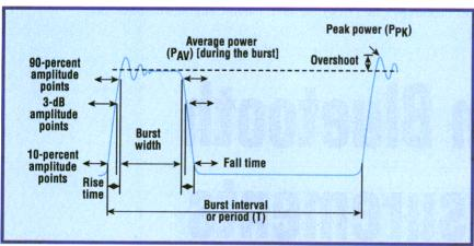
Bluetooth output-power measurements are performed in the time domain, based on these pulsed-signal characteristics.
