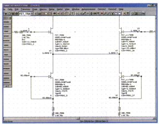
3. These DC bias configurations are for the diode section (a) and the PHEMT section (b) of the differential amplifier.
