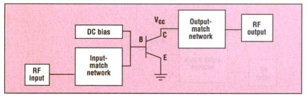
1. This block diagram shows the BJT in a common-emitter configuration, along with the DC bias and impedance-matching networks.
