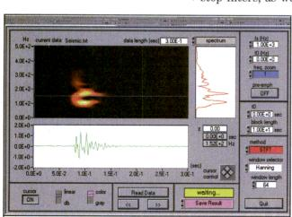
The JTFA software was used to analyze this seismic waveform for its power spectrum (right-hand plot) and its time response (lower plot).
