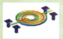
The current distribution and radiation pattern of a handset antenna modeled on IE3D
