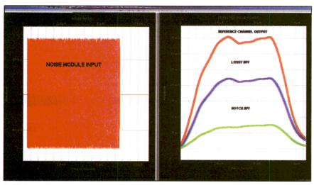
5. This modulated noise signal (left) was used to generate the simulated responses shown at the right for the three receiver channels.
