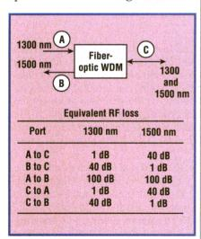
3. A wavelength division multiplexer has three portsa common port and two I/O ports.
