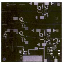
2. This photograph shows the millimeter-wave upconverter MCM, which includes some diagnostic subcircuits.
