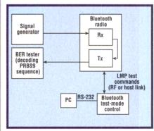
In this BER test setup, the Bluetooth DUT is placed in loopback mode with the BER tester. DUT. The output of the DUT's transmitter can then be routed to the BER tester for analysis. Provided with a PRBS 9 payload, the BER tester can determine the BER (Fig. 9).
