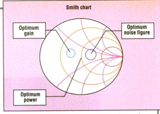
4. The optimal-load impedances for three different characteristics lie at different points on the Smith chart.
