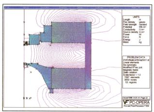
1. This axisymmetric model of the EIA klystron's magnetic circuit shows the lines of magnetic flux.
