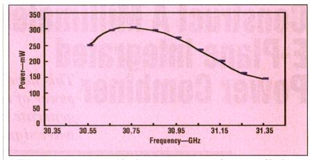
4. This graph shows the combined power output versus frequency of both Gunn diodes operating simultaneously.
