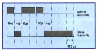
1. The Bluetooth TDD/frequency-hopping structure is based on 625- $\mu s$  time slots. asynchronous-connectionless (ACL) links. The SCO links are intended for the transmission of continuous streams of 64-kb/s audio. The standard supports pulse-code-modulation (PCM) encoded audio (using A-law or µm-law weighting) and continuous-variable-slope-delta (CVSD) modulation encoded audio. The ACL links are used for data transmissions.
