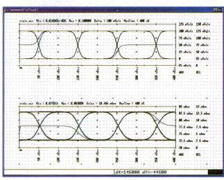
5. These eye diagrams were generated for the differential amplifier simulated at 10 Gb/s.
