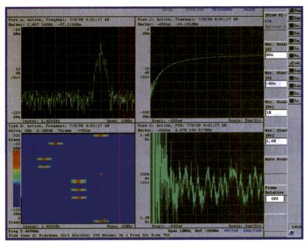
2. These four screens show the frequency spectrum, amplitude profile, modulation characteristics, and spectrogram of simulated Bluetooth signals.
